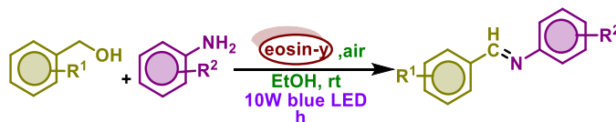
Figure 1. Visible light promoted synthesis of Schiff base from benzyl alcohol and aniline.
